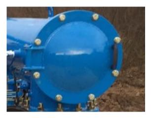
• FMA4000 filters use standard bolts and nuts on both side flanges instead of the previous system with the bolts welded to the filter housing. In this way, if one day to replace a bolt is required, it can be done easily.
